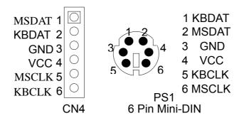
Figure 0-2 CN4 & PS1: PS/2 KB/Mouse Connector
